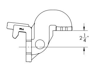
MATERIAL COMPOSITION LIFT-OUT FLANGE: ASTM A48 CAST IRON BASE GROMMET: NITRILE RUBBER DISCHARGE GASKET: ALL HARDWARE IS 304 STAINLESS STEEL
